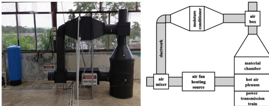
**Figure 2:** Depiction of the HARC<sup>2</sup>S located at the University of Puerto Rico at Mayagüez. (a) Side-view picture of the dehydration system. (b) Sketch of the system with identification of the major components.
