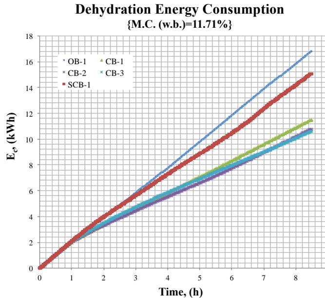
**Figure 3:** Depiction of the HARC<sup>2</sup>S dehydration cumulative energy consumption continually measured using a watt node 208/240 VAC 3-phase delta/bye kWh transducer-sensor (T-WNB-3D-240) and recorded with a HOBO (UX120) pulse data logger.
